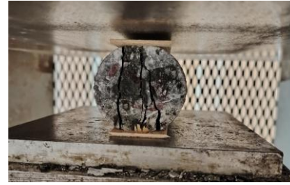
(b) Failure in a concrete cylinder after the split tensile strength test
