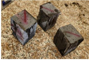
(a) Failure mode of the concrete cube after the compressive strength test
