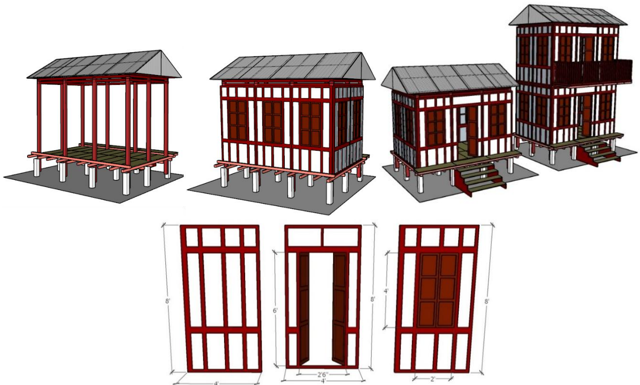
Figure 04. Proposed 4'x8' modular wooden panel and the growth of the incremental house (Source: Authors).
