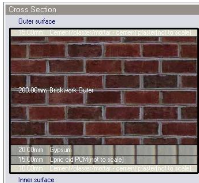
Figure 4. Clay brick wall + Capric Acid PCM + Gypsum.
