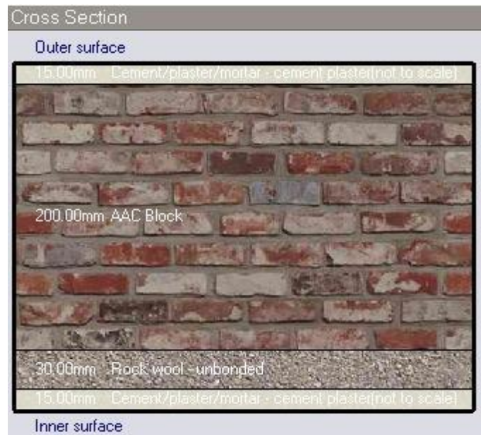
Figure 1. Conventional clay brick wall assembly without PCM.
