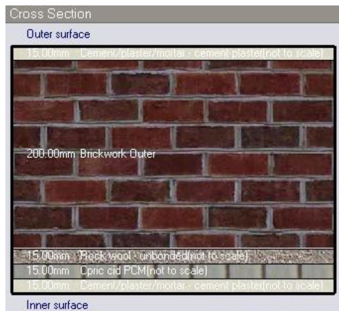
Figure 2. Clay brick wall with Capric Acid PCM.
