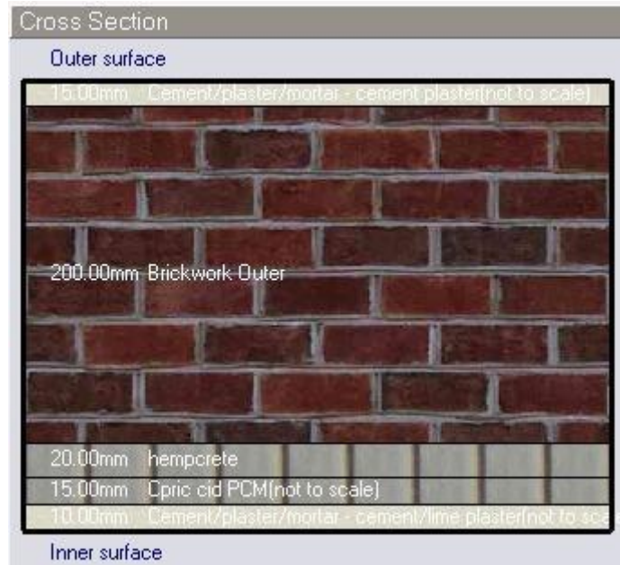
Figure 5. Clay brick wall + Capric Acid PCM + Hempcrete.
